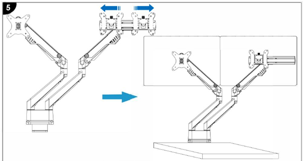
**Additional note:** Select the other 2 connection points on the monitor slider to further extend the range of the monitors.
